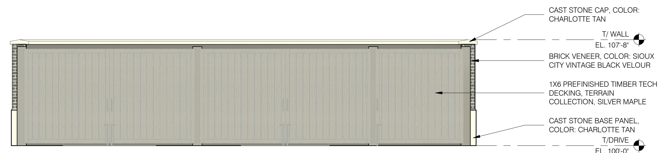
5 FRONT DUMPSTER ELEVATION SCALE: 1/4" = 1'-0"
